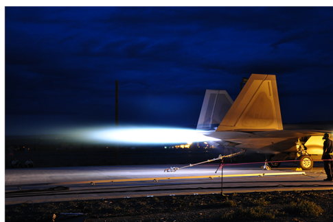
Fig. 1 a) Experimental setup schematic and b) photograph from F-22A Raptor test (ground array is along pavement edge).
