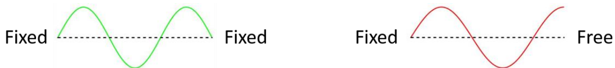
Figure 1. Third mode shape of a fixed-fixed string (left) and a fixed-free string (right).
