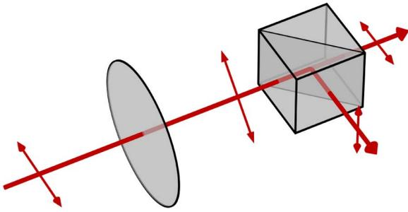
**Fig. 1.** Beamsplitting using an ideal half-wave plate and a polarizing beamsplitter. The beam entering on the left is horizontally polarized. After the polarization is rotated by the wave plate, a polarizing beamsplitter separates the horizontal and vertical components.
