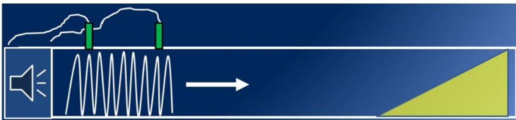
Figure 4: If microphones are spaced far apart relative to the wavelength, they detect a larger wavelength than is actually present.
