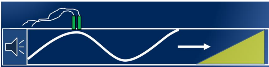
Figure 3: If microphones are spaced too closely relative to the wavelength, they can't detect wave amplitude differences.
