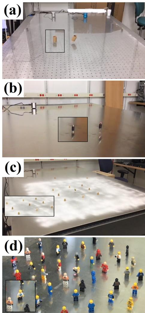
FIG. 7. (Color online) Photographs of time reversal focusing being used to knock over objects. The inset image, outlined in black, shows the undisturbed state. (a) A cardboard cylinder is knocked over on the glass plate. (b) An RCA adapter, (c) wooden cork (developer spray was applied to allow laser scanning), and (d) Lego minifigure are knocked over on the large aluminum plate.
