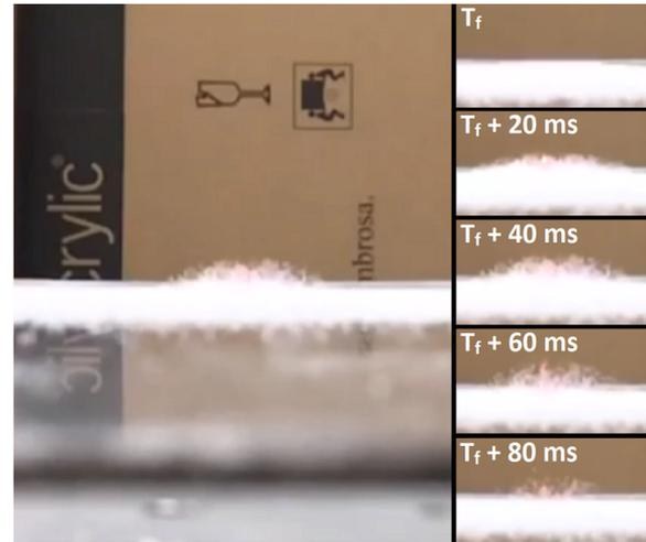
FIG. 6. (Color online) Photograph of salt jump visualization at the time of peak salt displacement (left) and snapshots at the time of focus and afterwards (right).
