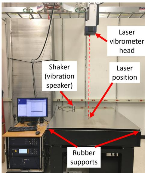
FIG. 1. (Color online) Photograph of experiment setup with a large aluminum plate. The shaker is mounted on the upper left corner of the plate.
