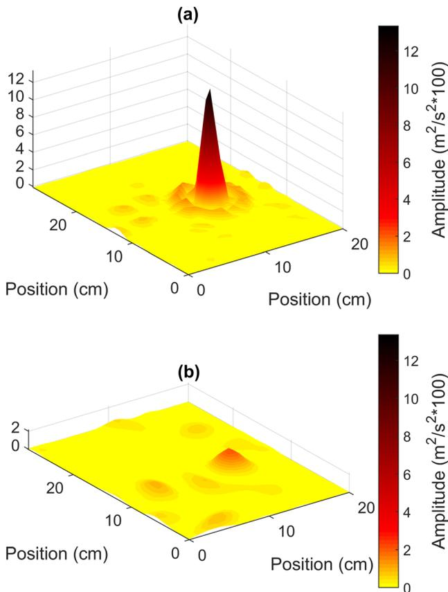
FIG. 4. (Color online) Spatial maps of the instantaneous energy at the time of peak time reversal focusing. (a) Glass plate. (b) Cardboard plate. Color denotes amplitude. The peak heights are to scale with respect to each other (meaning 2 units on the z-axis is the same for both plots).
