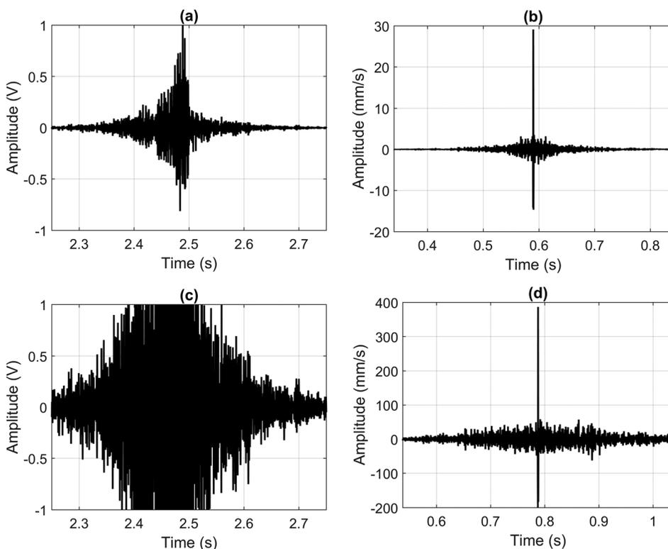
FIG. 3. Deconvolution time reversal (TR) signals obtained on the glass plate. (a) Deconvolution TR signal without clipping. (b) Deconvolution TR focal signal without clipping. (c) Deconvolution TR signal with 10 times clipping. (d) Deconvolution TR focal signal with 10 times clipping.
