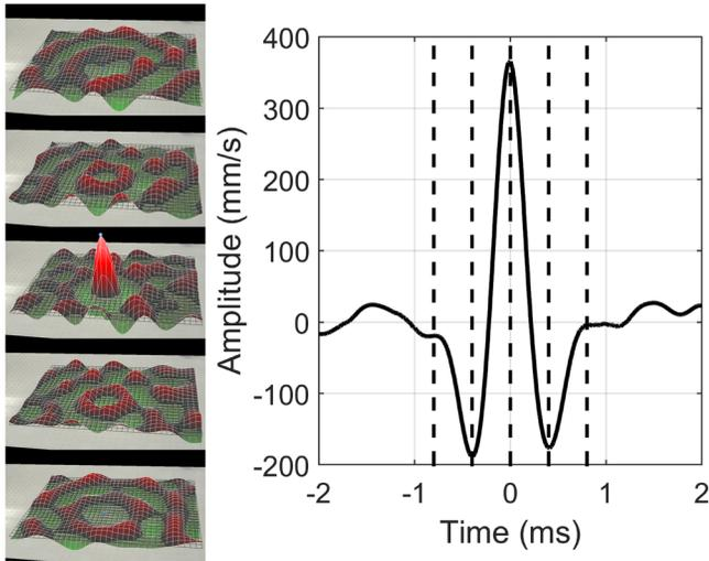
FIG. 5. (Color online) Evolution of the time reversal focusing over time. Spatial maps at different time intervals (left) and focal signal at focal location (right). Dashed lines indicate times corresponding to the spatial maps.
