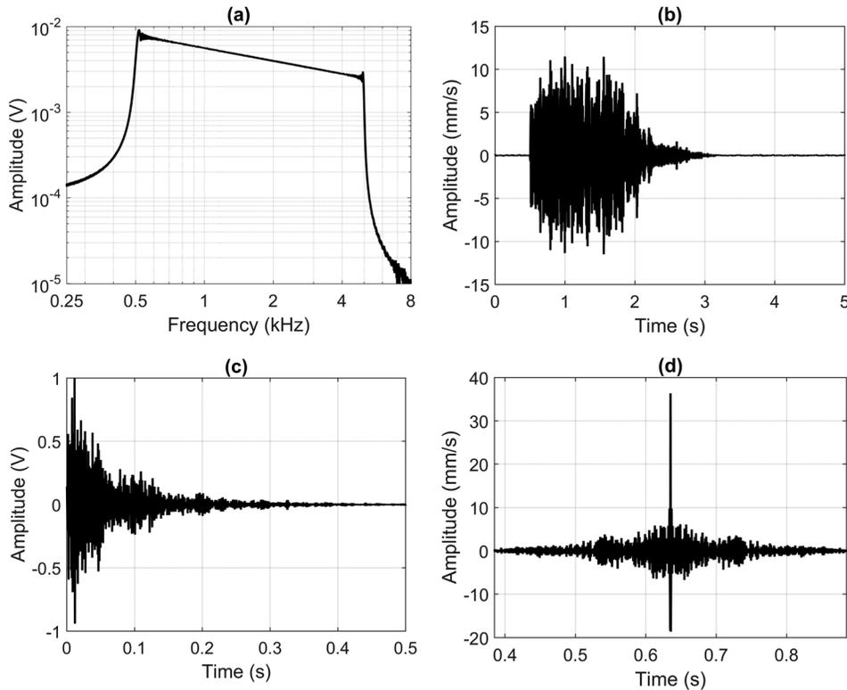
FIG. 2. Sample signals from a time reversal experiment. (a) Spectrum of the chirp signal,  $FFT\{s(t)\}$ , sent to the source. (b) Chirp response,  $r(t)$ , recorded by the laser vibrometer on the glass plate. (c) Impulse response,  $ir(t)$ , extracted from the cross correlation. (d) Focal signal,  $y_{TF}(t)$ , recorded by the laser vibrometer when the reversed impulse response is broadcast from the source.
