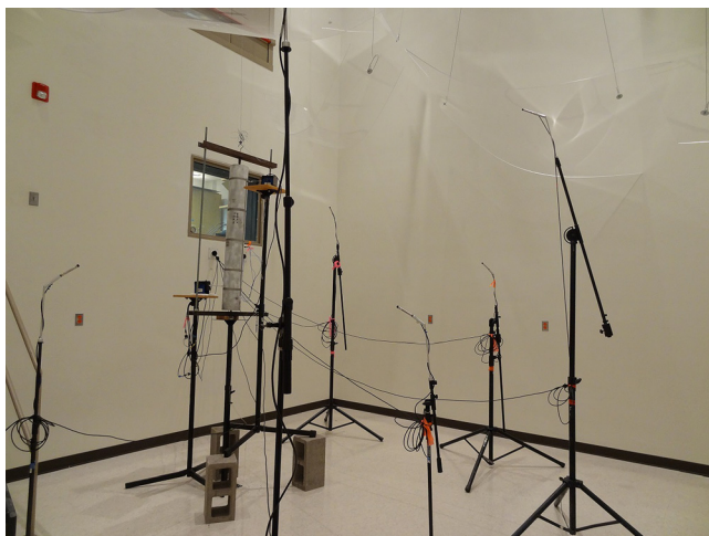
FIG. 11. (Color online) The experimental setup showing the cylindrical shell, shakers, and accelerometers, as well as the microphone placement.
