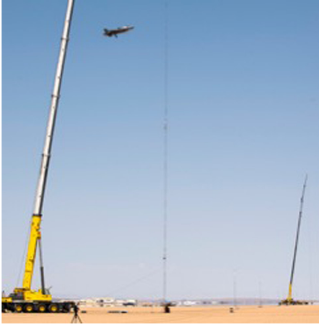
FIG. 1. (Color online) An F-35 flying between two cranes, each located 305 m (1000 ft) from the flight path of the aircraft. Microphones were hung from the 91.4 m cranes at multiple heights, with five heights having redundant 1/2 and 1/4 in. microphones.
