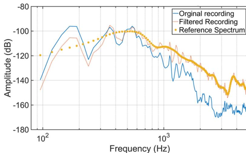
*Figure 2. Autospectra of the original, filtered, and reference recordings from 2007.*
