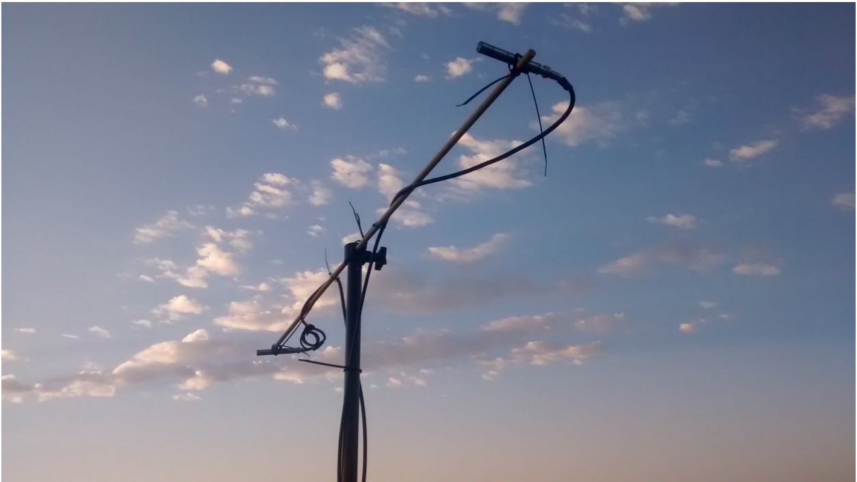
Figure 3. An example of the pressure measurement setup, with both microphones pointed towards the source.
