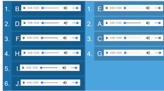
Figure 8: Screenshot of user interface for the random access (ordering) test. At the beginning of the test, all 15 sound samples are on the left. Subjects tap on sounds for playback and then drag and drop them to the right side, placing them in order from least to greatest (top to bottom) amount of perceived crackle.
