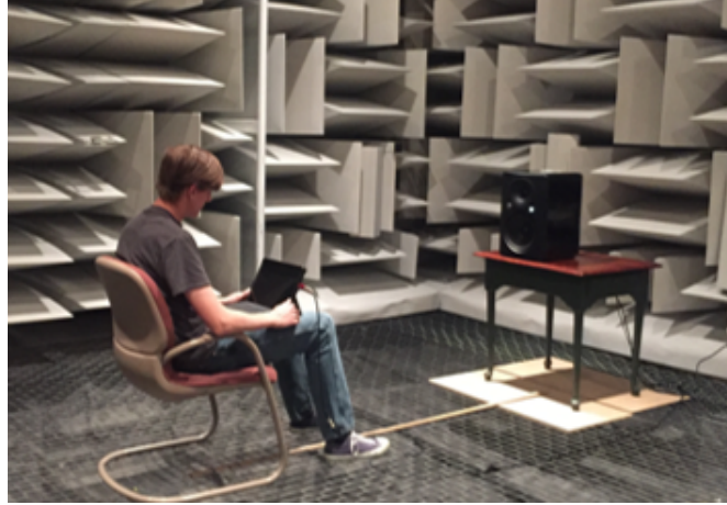
Figure 10: Listening test setup in BYU's anechoic chamber.
