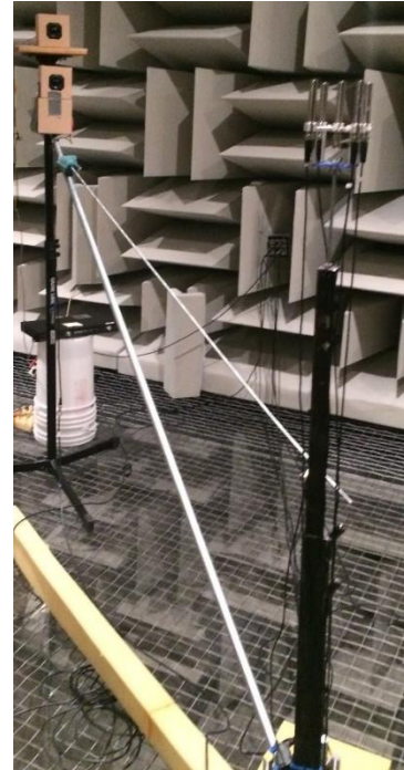
Figure 16: A two-speaker setup in an anechoic chamber. The speaker on the arm rotates, so the angle of rotation is the same as the angle of separation between the speakers.
