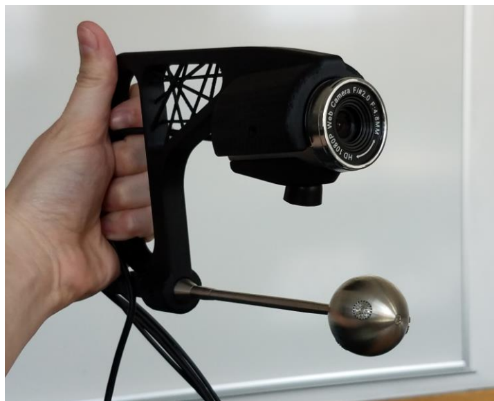
Figure 1. The 3D printed holder with the web camera and the spherical microphone probe.
