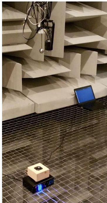
Figure 4. Experimental setup for determining the precision and accuracy of the azimuthal and elevation angles consisting of a white noise sound source (speaker) and the 3D handle unit attached to a 3D scanning system in the anechoic chamber.
