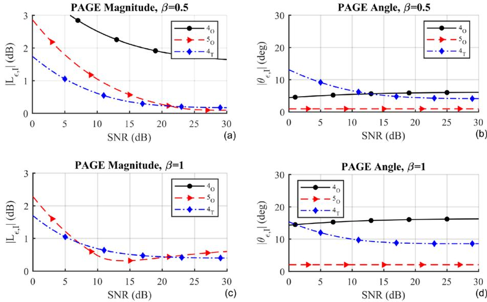
FIG. 11. (Color online) Probe comparison of bias errors for a monopole source at two distances ( $\beta = 0.5$  and  $\beta = 1$ ) with contaminating uncorrelated noise using the PAGE method. Both magnitude and direction errors are shown for both cases. In (c) the bias errors for  $4_O$  are greater than 3 dB for all SNR values below 30 dB.
