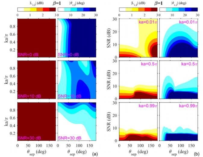
FIG. 8. (Color online) Bias errors for a monopole source located a distance  $r = a[\beta = (ka/kr) = 1]$  from the probe center with contaminating correlated noise using (a) the traditional method and (b) the PAGE method.
