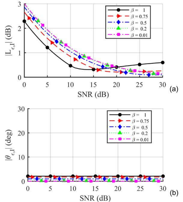
FIG. 5. (Color online) PAGE method bias errors in (a) the magnitude and (b) the direction of the active intensity calculated for a monopole source with uncorrelated contaminating noise using a five-microphone orthogonal probe, averaged across angle of incidence.
