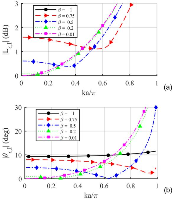
FIG. 4. (Color online) Traditional method bias errors in (a) the magnitude and (b) the direction of the active intensity calculated for a monopole source with uncorrelated contaminating noise using a five-microphone orthogonal probe. Results are averaged across angle of incidence. In (a) the bias errors for  $\beta = 1$  are greater than 3 dB for all values of  $ka$ .
