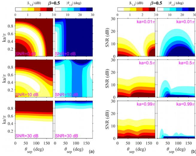
FIG. 7. (Color online) Bias errors for a monopole source located a distance  $r = 2a[\beta = (ka/kr) = 0.5]$  from the probe center with contaminating correlated noise using (a) the traditional method and (b) the PAGE method.
