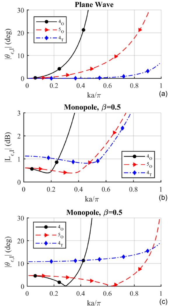
FIG. 10. (Color online) Bias errors for different probe geometries with contaminating uncorrelated noise using the traditional method. Only cases where the different probe geometries exhibit marked differences are pictured. The angular error for a plane-wave source with uncorrelated noise is given in (a), while (b) shows the magnitude error and (c) shows the angular error for a monopole source.
