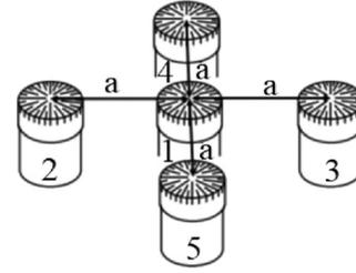
FIG. 1. A five-microphone orthogonal probe. The microphones are numbered 1 to 5, and in the  $x$ - $y$  plane of the probe—where  $\hat{x}$  goes from 1 to 3 and  $\hat{y}$  goes from 1 to 4—have positions  $(0,0)$ ,  $(-a,0)$ ,  $(a,0)$ ,  $(0,a)$ , and  $(0,-a)$ , respectively.
