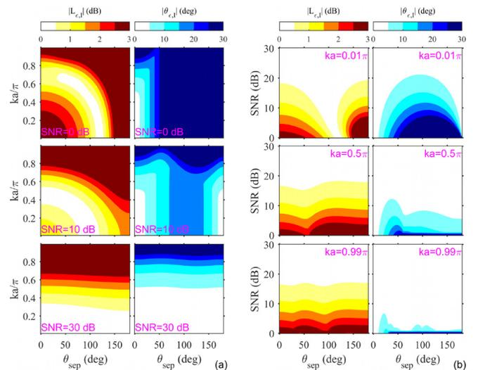
FIG. 6. (Color online) Bias errors for a plane-wave source with contaminating correlated noise using (a) the traditional method and (b) the PAGE method.
