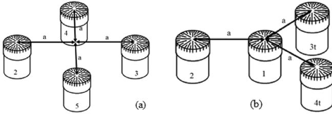
FIG. 9. Two alternate probe geometries that can be used to calculate intensity. The four-microphone orthogonal probe (a) is referred to as  $4_O$  and the four-microphone triangular probe (b) is referred to as  $4_T$ . The five-microphone orthogonal probe in Fig. 1 is referred to as  $5_O$ . Note there is no microphone 1 for  $4_O$ , and are numbered 2 through 5 to match the numbering for  $5_O$ .
