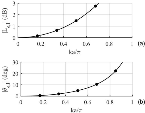
FIG. 2. Traditional method bias errors in (a) the magnitude and (b) the direction of the active intensity calculated for a plane-wave source with uncorrelated contaminating noise using a five-microphone orthogonal probe. The bias errors are plotted as a function of only  $ka$  because the results are independent of SNR and are averaged across all possible angles of incidence.
