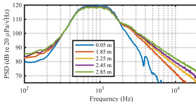
Figure 1. Spectra at different distances along the plane wave tube.
