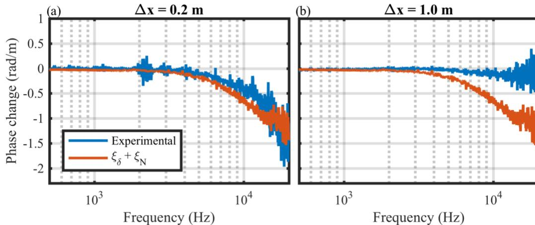
**Figure 3. Comparison of experimentally determined  $\partial\theta/\partial x$  to  $\xi_N + \xi_\delta$ .**
