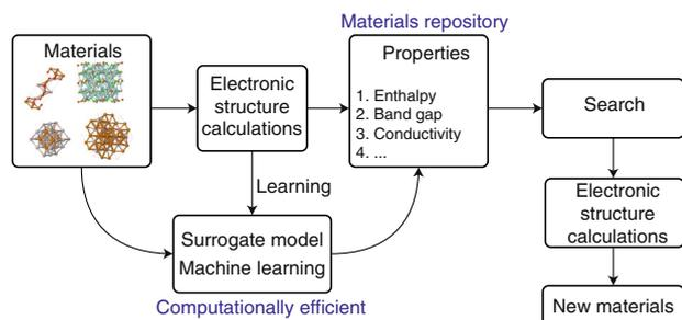
**Fig. 1** The accelerated high-throughput approach. Candidate structures and properties are generated by surrogate machine-learning models based on reference electronic structure calculations in a materials repository. Selected structures are validated by electronic structure calculations, preventing false positive errors
