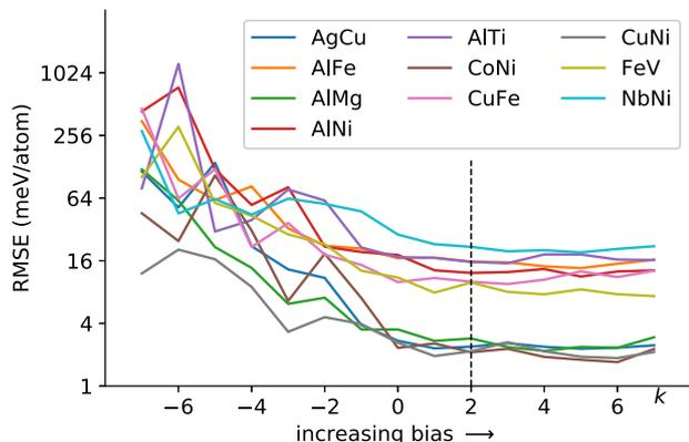
**Fig. 4** Influence of biased training and validation sets. Shown are the root mean squared errors (meV/atom) as a function of training and validation set composition obtained using MBTR + KRR model. See main text for discussion
