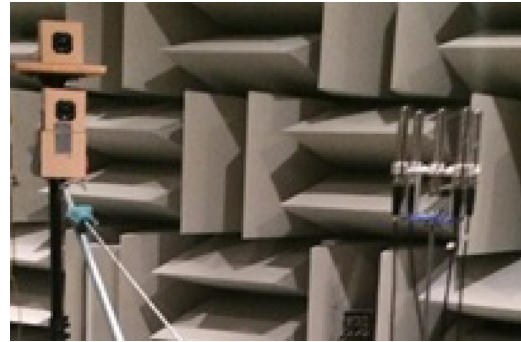
FIG. 7. (Color online) Experimental setup. The source loudspeaker location is fixed, while the additive noise loudspeaker is on a rotating arm to have variable angular separation.
