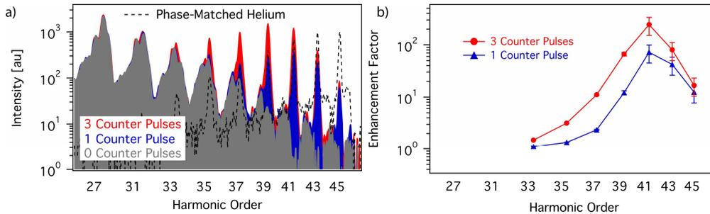
Fig. 9. (a). Observed harmonic emission from argon for no (gray), one (blue), and three (red) counterpropagating pulses. Phase-matched emission from 100 torr helium (dashed black) is included for comparison. (b). Enhancement factor as a function of harmonic order, for one (blue) and three (red) counterpropagating pulses [58].
