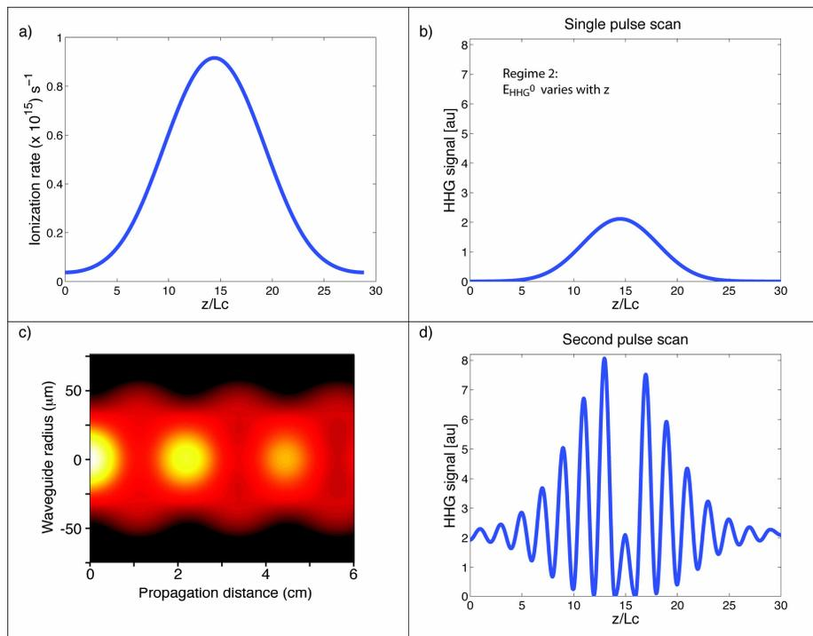
Fig. 7. Simulation of the HHG output when a) the ionization rate varies due to mode beating, for b) the scan of a single counterpropagating pulse, and d) the scan of a second counterpropagating pulse when the first is held fixed at  $z/L_C=15$ . The model assumes an interaction between the two lowest order coupled modes, which induce a periodic variation of intensity, shown in c).
