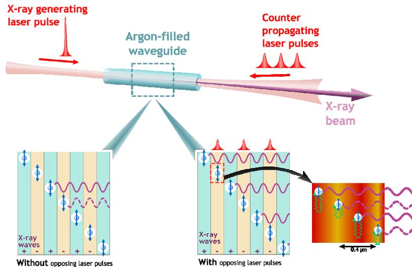
Fig. 1. Schematic for HHG in a hollow waveguide, illustrating the use of counterpropagating light to compensate for phase mismatch using all-optical quasi phase matching [1].
