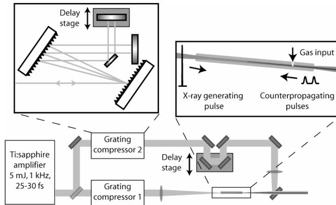
Fig. 2. Experimental setup for measuring the in-situ coherence length and implementing all-optical QPM using counterpropagating pulses.
