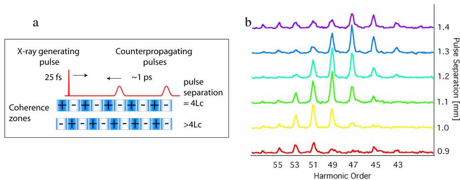
Fig. 11. Tuning the selectivity of all-optical QPM using two counterpropagating pulses, by varying their separation. The effective pulse widths of each pulse was  $\sim 300 \mu\text{m}$ . A schematic illustrating this effect is shown in a). Enhancement occurs when the pulse separation is  $2^N L_C$ . Selectivity improves when  $N > 1$ . HHG spectra from argon, in b), show the shift of the enhancement with harmonic order as the separation between the pulses is varied.
