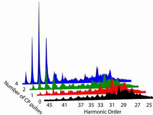
Fig. 10. All-optical QPM of HHG in argon, with a train of up to four counterpropagating pulses.
