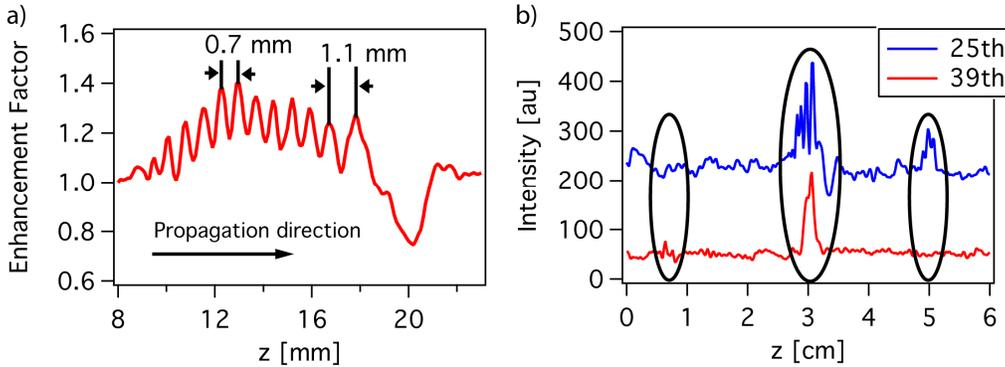
Fig. 4. Spatial variations in the local coherence length of HHG with propagation distance in a hollow waveguide. (a). Loss mechanisms lead to an increasing coherence length with propagation distance. (b). Modebeating causes the harmonic emission to be localized in the waveguide at a periodicity of  $\sim 2.2$  cm.
