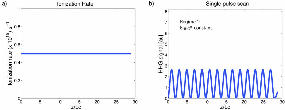
Fig. 6. Simulation of a scan of counterpropagating pulse when the strength of harmonic field and  $L_C$  do not vary along propagation. a) A constant ionization rate with propagation and b) the variation in the intensity of the detected harmonic signal for the scan of a single counterpropagating pulse, showing coherent ringing.
