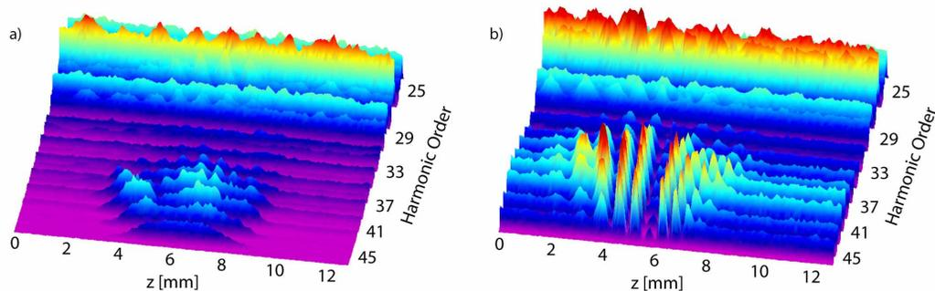
Fig. 8. Harmonic spectra observed in 8 torr argon as a function of the position of the overlap region,  $z$ , between the forward- and counterpropagating pulses. a) A single counterpropagating pulse is scanned through the interaction region, showing little coherent ringing. b) A second counterpropagating pulse is scanned through the interaction region, while the first remains stationary at  $z \approx 6$  mm. Here, strong coherence is observed.
