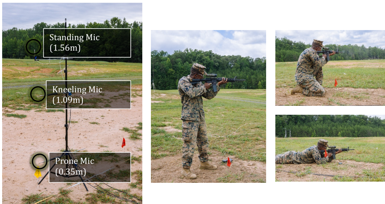
Figure 3. Example of microphone stand with three different heights. Shooters at three different heights shown at the right.
