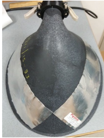
Figure 8: A photo of the Pyrotek constrained layer damping material applied to the bowl.
