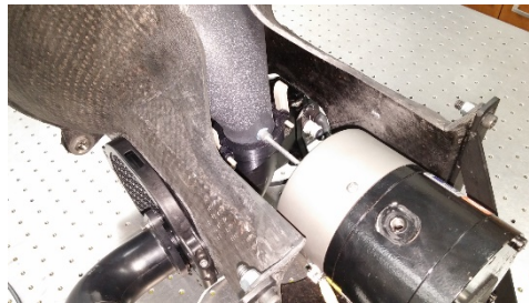
Figure 3: A photo of a shaker attached to the bottom of the bowl. This is where the bowl was excited for scanning laser Doppler vibrometer measurements.
