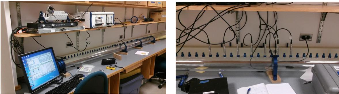
**Figure 1. Photos of experimental setup. (Left) The DAQ is connected to the speaker system (on the left end of the plane wave tube), as well as the National Instruments Hardware on the shelf. The anechoic termination is visible on the far right of the image. (Right) Seven microphones spaced 10 cm apart, placed roughly in the middle of the tube. The middle microphone is not phase-matched, but the remaining six are phase-matched.**
