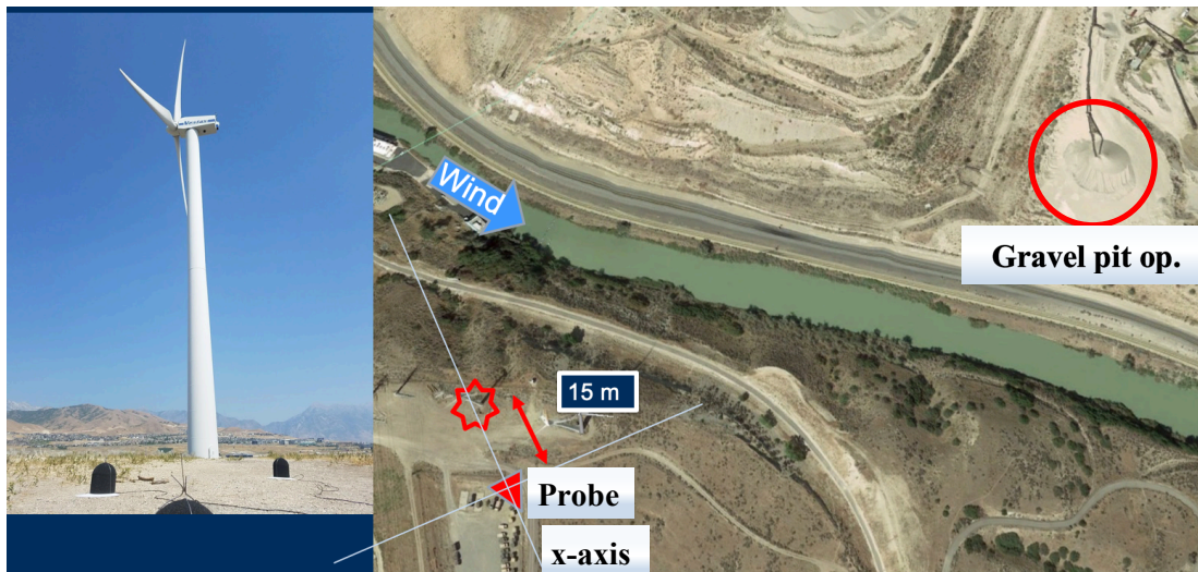
Figure 8. Vestas V47/660 wind turbine experiment setup. The red asterisk shows the wind turbine location, and the triangle the probe location, the thin-gray line going downwards in the picture shows the zero degree axis. The approximate location of the gravel mining operation is also shown.
