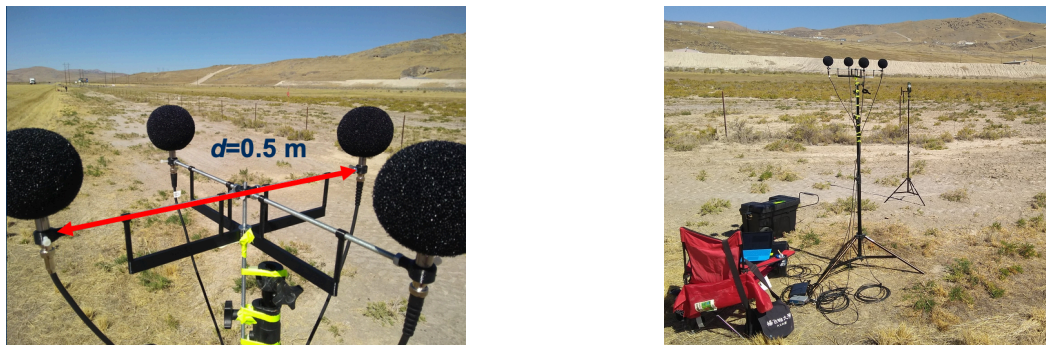
Figure 2. Left: Intensity probe, with 0.5 m between orthogonal microphone pairs. Right: The probe location with the rocket test site in the upper part of the picture
