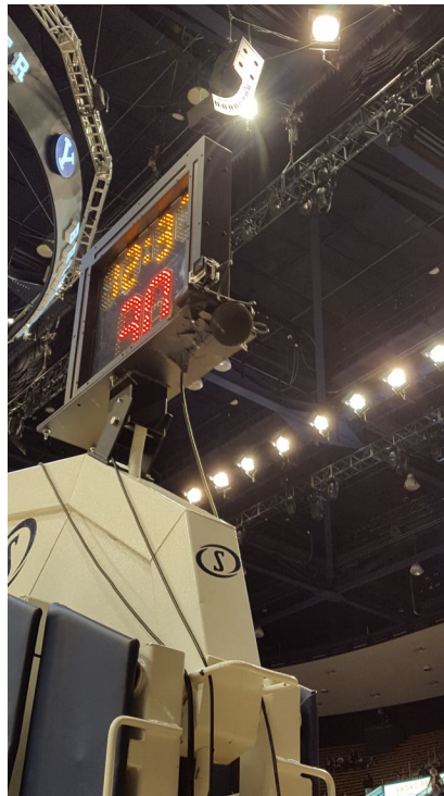
Figure 1. The typical microphone setup used for basketball games.
