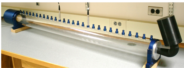
Fig. 3—The impedance measurement setup, with a resonator attached to the end of an impedance tube. Two microphones are mounted in the impedance tube, and a speaker is mounted on the end opposite the resonator.
