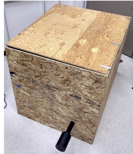
Fig. 8—Test setup for resonator-enclosure coupling, with resonator A attached to the side of a plywood enclosure.
