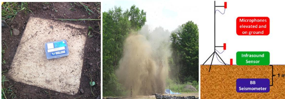
Figure 8- (Left) Buried soundproof box housing a microphone to detect seismic-acoustic coupling. (Middle) One of the six explosions from the second test (Pad 2)- Photo courtesy of Jacopo Taddeucci. (Right) A schematic of the sensor configuration.
