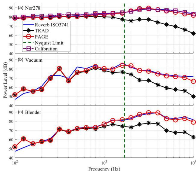
Fig. 3. (Color online) One-third octave sound power spectra in dB re 10 pW for (a) a Nor278 reference sound source, (b) a handheld vacuum cleaner, and (c) a household blender.
