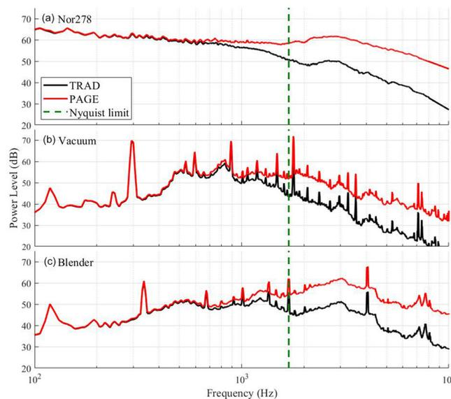
Fig. 2. (Color online) Narrowband intensity-based sound power spectra in dB re 10 pW for three sources with both TRAD and PAGE processing: (a) Nor278 reference sound source, (b) handheld vacuum cleaner, and (c) household blender. The spatial Nyquist frequency,  $f_{\text{Nyq}}$  is marked by a dashed vertical line.
