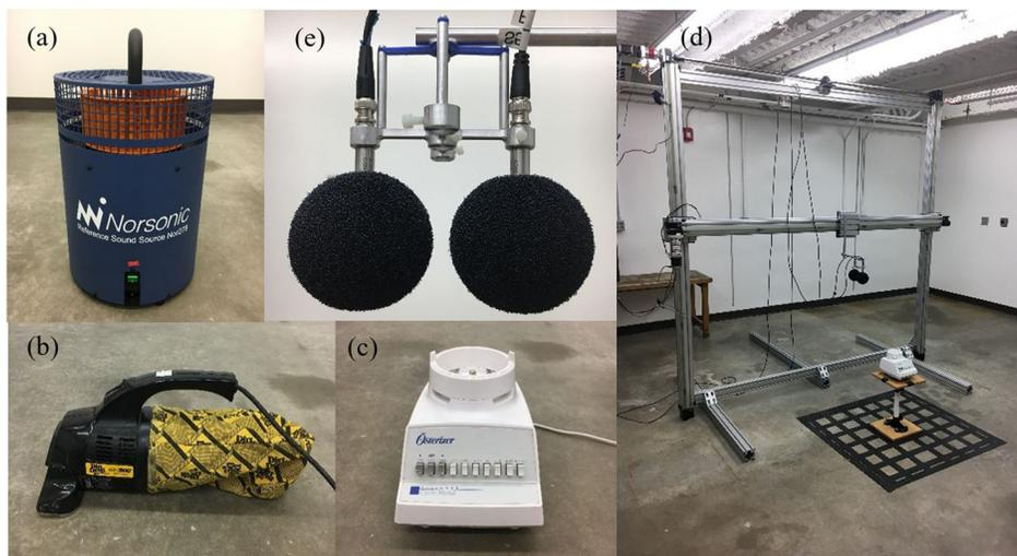
Fig. 1. (Color online) (a) Norsonic Nor278 reference sound source. (b) Handheld vacuum cleaner. (c) Household blender. (d) Experimental setup consisting of a 7 × 7 grid marking the location of the base of 1 m<sup>3</sup> control surface, a source in the center of the control surface cube, a gantry system, and a two-microphone probe. (e) Microphone probe with two phase-matched 1/2 in. G.R.A.S. 46AE microphones spaced 4 in. apart.
