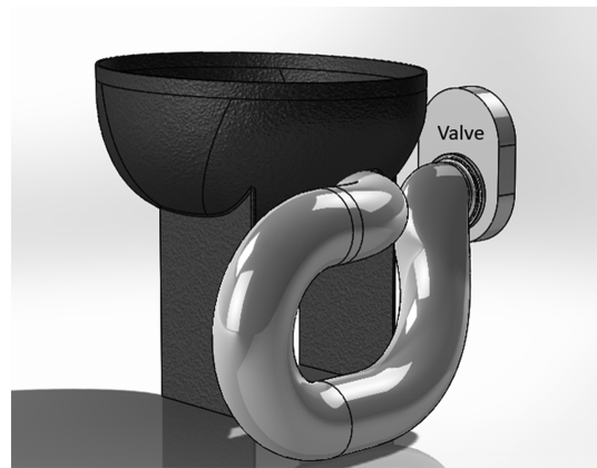
Fig. 18—Notional diagram of how an insert may fit behind the toilet, i.e., back-only insert.
