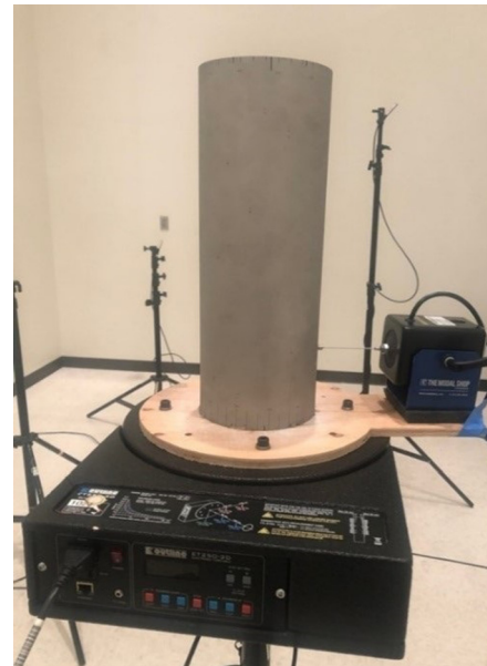
FIG. 10. (Color online) Setup of a mounted cylinder on a turntable with a shaker to excite the cylinder. The microphones and reverberation chamber used for ISO 3741 are seen in the background.
