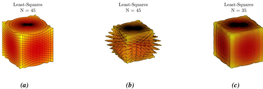
**Figure 5:** *Least-Squares spherical harmonic expansion of a unit cube on a  $5^\circ$  and  $2.5^\circ$  grid. (a) The  $N = 45$  expansion evaluated on the original  $5^\circ$  grid. (b) The  $N = 45$  expansion evaluated on a finer  $2.5^\circ$  grid. (c) The  $N = 35$  expansion evaluated on a finer  $2.5^\circ$  grid.*
