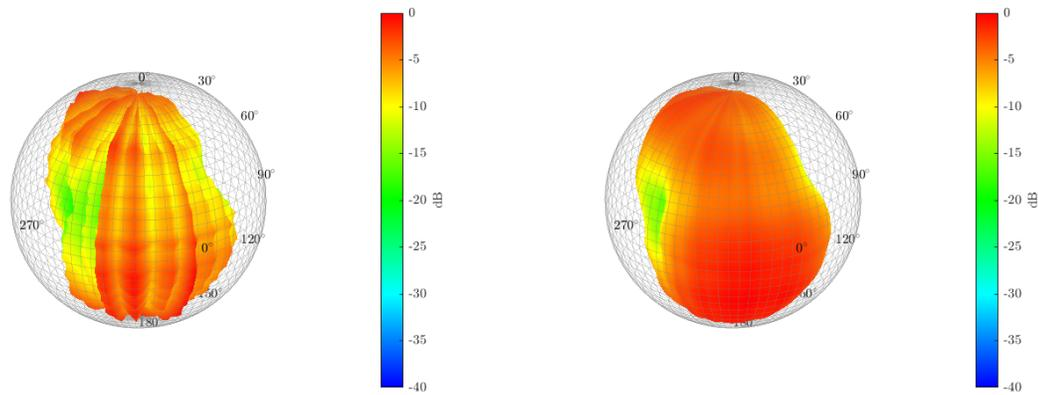
(a) *The autospectral balloon.*(b) *The frequency response balloon.***Figure 2: Flute Directivity at 311 Hz (E♭ 4).**
