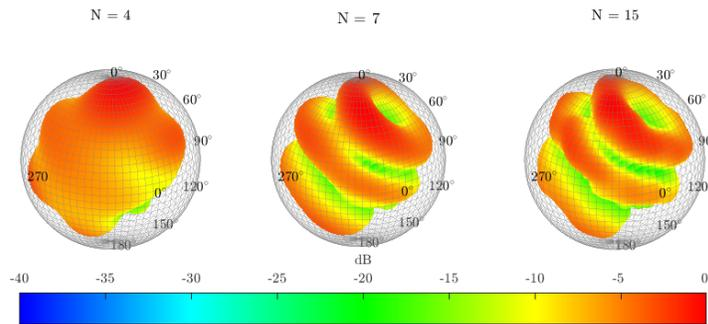
**Figure 7:** Bassoon directivity balloon at 550 Hz over varying expansion degrees.
