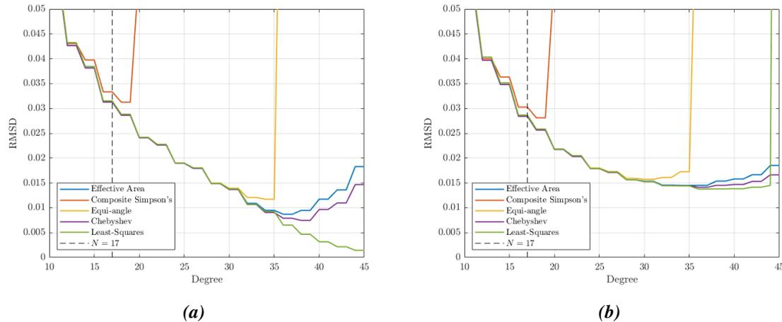
**Figure 4:** *The RMSD between the spherical harmonic expansion over  $5^\circ$  and  $2.5^\circ$  grids, and known values on the grids, plotted over expansion degree. The spherical harmonic expansion used is the same in both 4a and 4b; however, the finer grid used in 4b allows for a check of whether the interpolated values between sampling points remains valid.*
