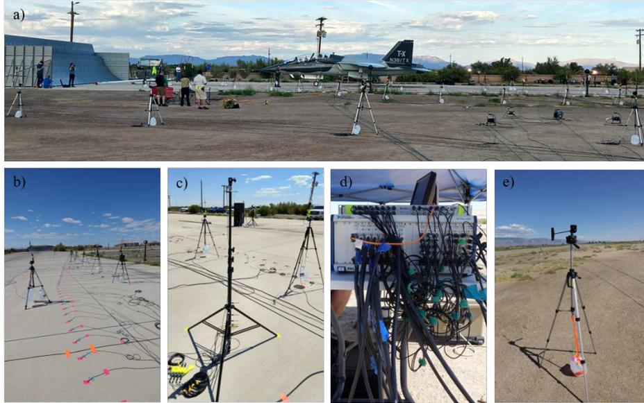
**Fig. 2** Images of T-X measurement layout at Holloman Air Force Base, New Mexico: a) tied-down aircraft with 38.1 and 19.2 m (125' and 63') arcs and maintainer mics visible, b) imaging ground array and maintainer mics facing downstream, c) 130° crackle station facing a loudspeaker located at the MARP, d) imaging array data acquisition unit, and e) Kestrel weather station located at 57.2 m (187.5') along the 70° radial.
