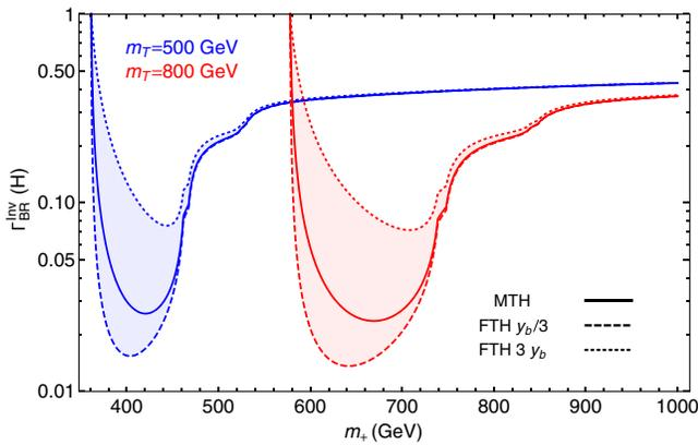
FIG. 2. Branching fraction of the twin sector Higgs to twin states as a function of its mass for the MTH (solid curves) and FTH (dashed and dotted curves) models. The blue (red) curves correspond to a mirror top mass of 500 (1000) GeV. In the FTH model the twin bottom Yukawa varies from one third the SM value (dashed line) to three times the SM value (dotted line).
