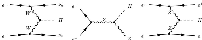
FIG. 5. Dominant Higgs production mechanisms at lepton colliders.
