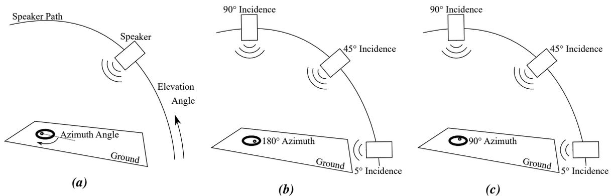
**Figure 3:** Schematic sketch of the anechoic chamber test setup, including (a) definition of the elevation and azimuthal angles. The ground board location was adjusted to place the microphone at the same location for each test, with azimuthal angle of (b)  $180^\circ$ , and (c)  $90^\circ$ .
