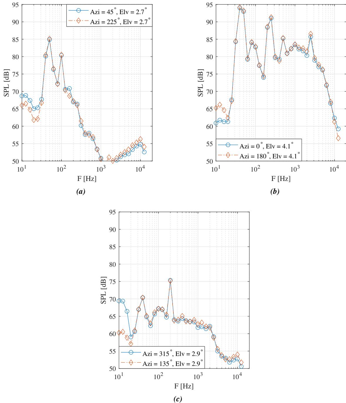
**Figure 12:** The spectra for two oppositely-oriented embedded microphones during a level flight of an S-76D Helicopter flying at 100 kts for (a) approach, (b) pass-by, and (c) departure.
