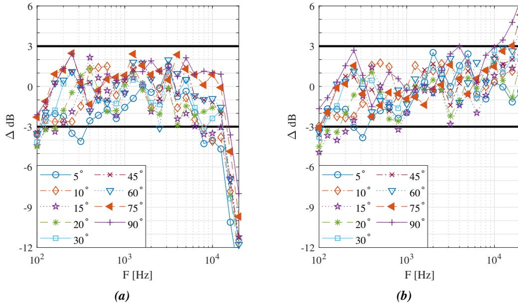
**Figure 8:** The differences (re: free-field) when the configurations were placed on plywood over three inches of sand and oriented at  $0^\circ$  azimuth relative to the sound source for (a) inverted and (b) embedded microphone.
