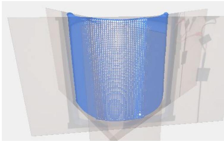
Figure 3: Example of stitched sections taken over the surface of the TR curved plate to measure the full complex surface velocity response, as seen in the SLDV software with scan points highlighted.
