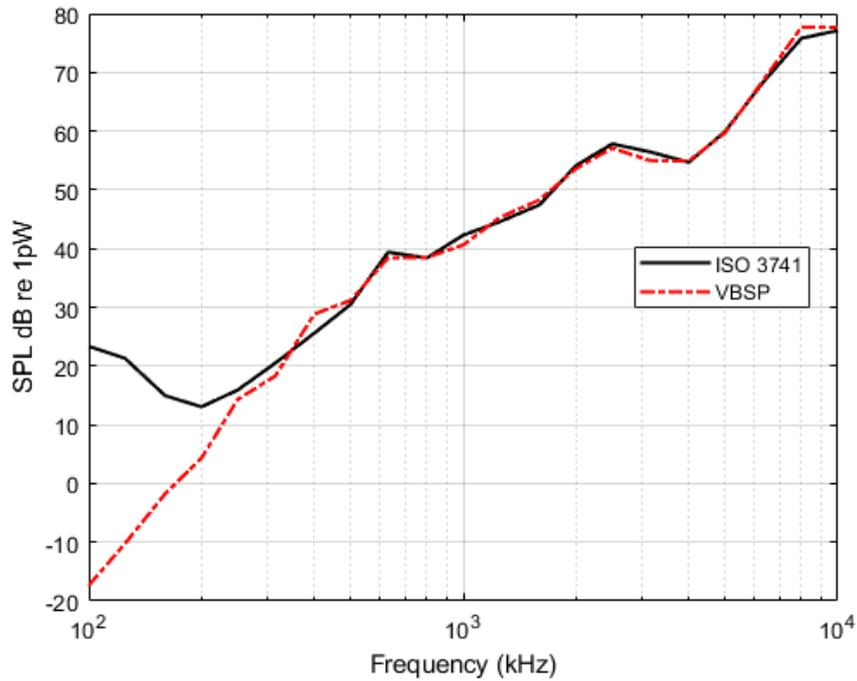
Figure 8: Results of the sound power measurements of the WR curved plate using the VBSP method (SLDV) compared to the ISO 3741 standard results.
