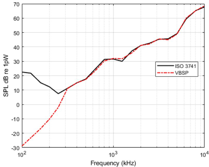
Figure 7: Results of the sound power measurements of the TR curved plate using the VBSP method compared to the ISO 3741 standard results.
