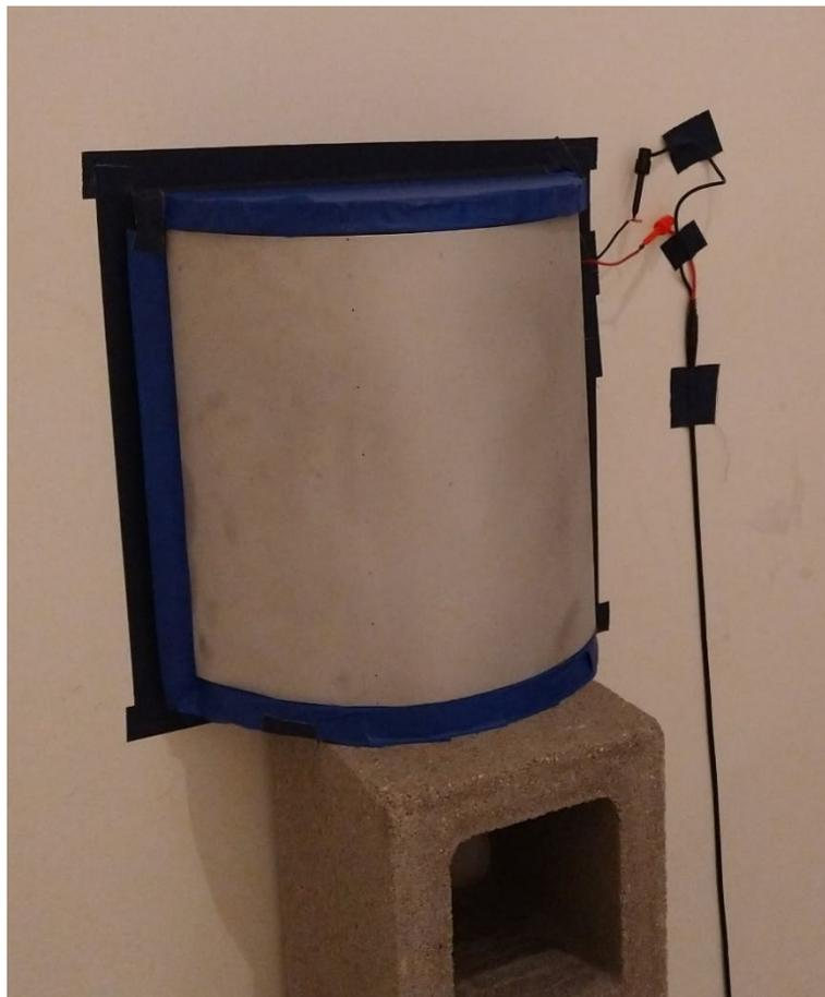
Figure 1: Setup of the TR curved plate in a reverberation chamber with the wall of the reverberation chamber acting as a baffle. The MR and WR curved plates were setup in the same manner shown.
