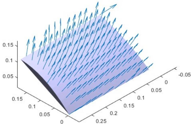
Figure 5: Example plot of unit normal vectors that are computed and placed on the surface of a curved plate. These vectors are obtained by processing geometry data from the SLDV.
