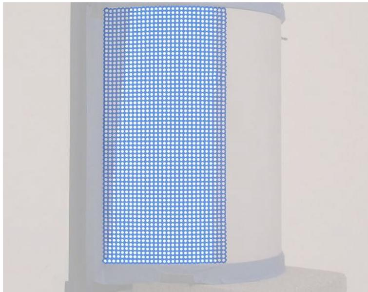
Figure 2: Example of one scan section taken over the surface of the TR curved plate to measure complex surface velocities, as seen in the SLDV software with scan points highlighted.
