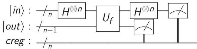
Fig. 3. Schematic for the quantum algorithm solving Simon's problem. Slashes on the horizontal lines with a number indicate a register of that many qubits. The  $n$ -qubit register is referred to as the input register and the  $(n-1)$ -qubit register as the output register. The lines at the bottom are an  $n$ -bit classical register.
