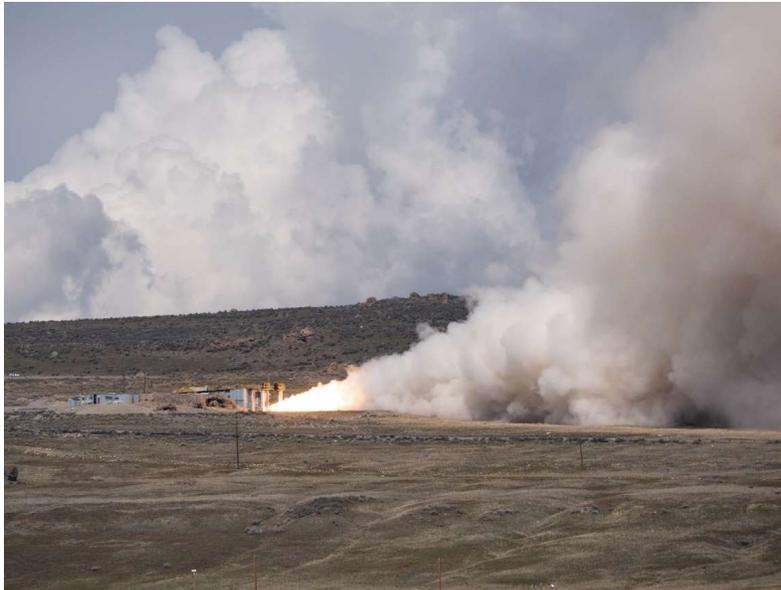
*Figure 2. Firing of the GEM 63 motor at the NGIS facility.*
