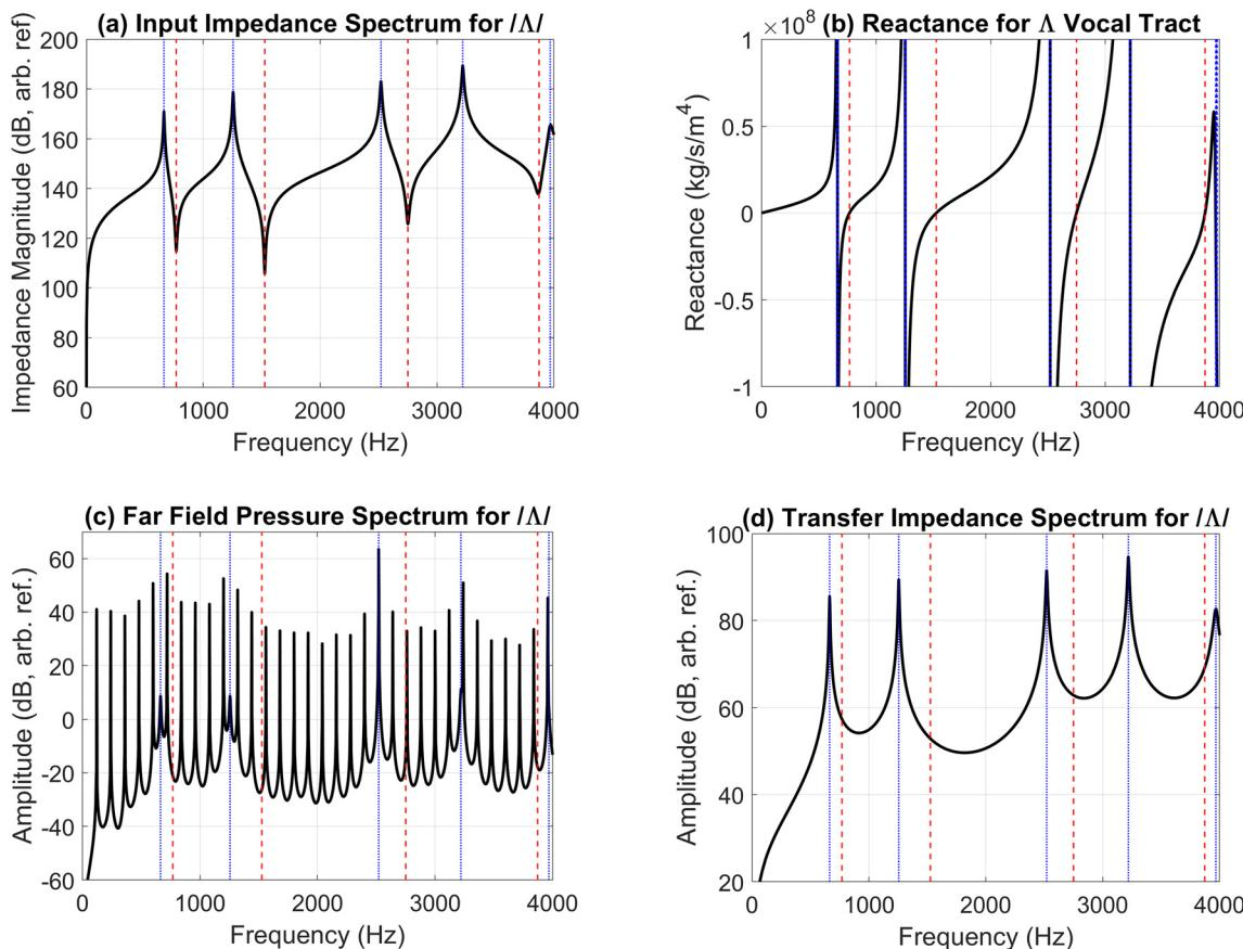
FIG. 6. (Color online) (a) Input impedance magnitude as a function of frequency for the phoneme /ʌ/. (b) Reactance of the input impedance for the phoneme /ʌ/. (c) Far field pressure radiation as a function of frequency for the phoneme /ʌ/. (d) Transfer impedance magnitude as a function of frequency for the phoneme /ʌ/. The blue dotted lines denote the peak frequencies of the input impedance and the red dashed lines correspond to positive-slope, zero crossings of the input reactance.
