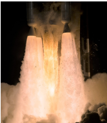
FIG. 6. (Color online) The Atlas V-541 launch of the Mars Perseverance Rover in March 2020. The liquid core-stage engine plumes show clear signs of overexpansion, whereas the structure of the outer solid booster plumes is obscured by burning aluminum particles. Photo courtesy of NASA.
