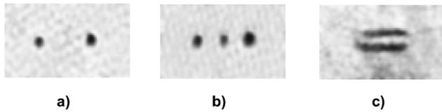
FIG. 4. Bose-Einstein condensates in time-averaged potential optical traps. Patterns with two (a) and three (b) points and a double sheet (c) are shown. The absorption images are taken along the axis of the laser beam, with resonant probe light. The frame size is  $200 \mu\text{m} \times 120 \mu\text{m}$ .
