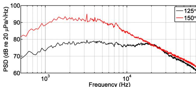
Fig. 2. (Color online) Power spectral densities (PSD) of the over-expanded Mach-1.8 jet at  $75 D_j$ .
