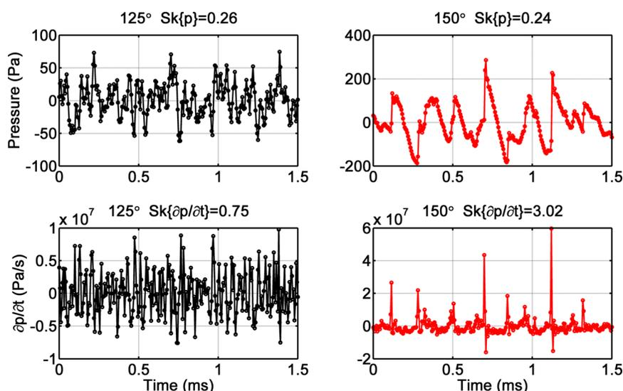
Fig. 3. (Color online) Waveform and time derivative segments for the Mach-1.8 over-expanded jet at  $75 D_j$  at  $125^\circ$  and  $150^\circ$ . Skewness values for the entire waveforms are also provided.
