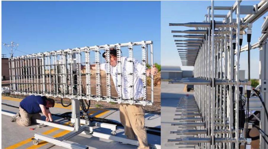
Fig. 2—Pictures of the rig holding a 5 x 18-microphone array. The rig is movable along the track and the physical center can be adjusted from 0.9 to 2.1 m (3 to 7 ft) from the ground.
