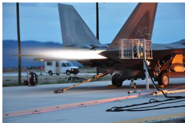
Fig. 1—The F22 Raptor tied down to the run-up pad with the 90-microphone array shown.
