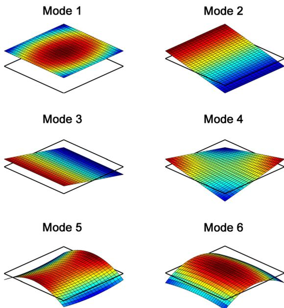
FIG. 1. (Color online) Acoustic radiation mode shapes.
