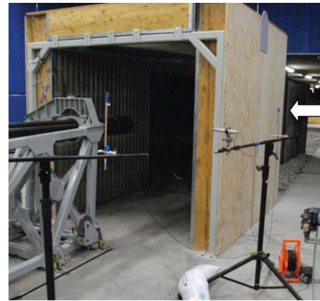
Fig. 11—Picture of the muffler built around the 30-mm gun, including microphones used for final measurements. The arrow is pointing at the microphone that recorded the data in Fig. 12.
