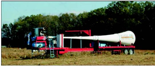
FIG. 1. (Color online) Photograph of the U.S. Army Research Laboratory's Mobile Acoustic Source (MOAS).
