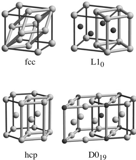
FIG. 3. Two real examples of three-dimensional superstructures. The  $L1_0$  structure (top right) is a doubled superstructure derived from the fcc lattice (top left). The  $D0_{19}$  structure (bottom right) is a quadrupled superstructure derived from an hcp parent multilattice (bottom left).
