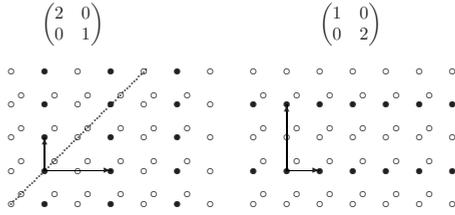
FIG. 5. Two equivalent multilattices. Though the bases are different, the first multilattice can be transformed into the second by a reflection about the line  $x-y=0$ . (Note that a  $90^\circ$  rotation is *not* a symmetry of the multilattice but the reflection is.)
