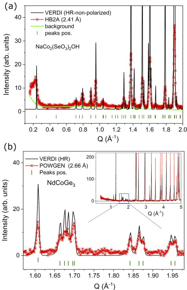
**FIG. 6.** Comparison of low- $Q$  coverage and  $Q$ -resolution of VERDI with HB2A (a) and POWGEN (b) instruments for two case studies involving magnetic orders with large magnetic unit cells or incommensurate propagation vectors. The relative intensities between different datasets are not reflecting the actual counting rates but are scaled for an easy comparison of the peak profiles.
