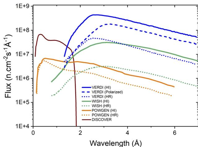
**FIG. 1.** Flux at the sample position against wavelength comparing VERDI (STS), WISH (ISIS-TS2), POWGEN (SNS), and DISCOVER (SNS). HI is high intensity and HR is high resolution instrument configurations.
