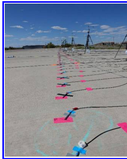
Fig. 1. Top. Schematic of the 120-microphone imaging array used for the analyses of this paper. Bottom. Images of the physical setup. On the left is the aircraft with microphones from different arrays seen on tripods. On the right, the microphones forming the imaging array are seen taped to the concrete runway.
