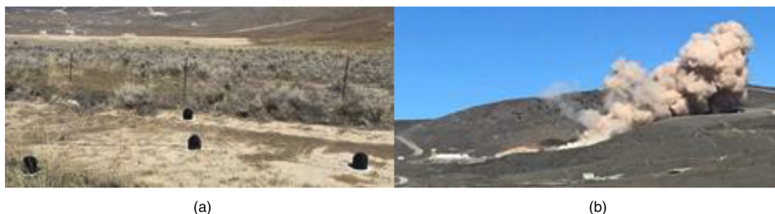
FIG. 4. (Color online) Experimental setup for measuring a static rocket booster firing, with a booster in the far distance (a). The firing of the booster is also shown (b).
