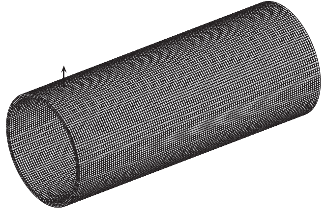
FIG. 10. Illustration of the cylinder mesh and the drive point location.
