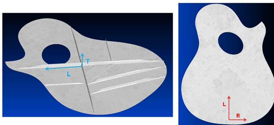
Fig. 2. (Color online) Finite element meshes shown from the (right) top and (left) bottom. The material directions are separately indicated for (right) the top plate and (left) the braces.
