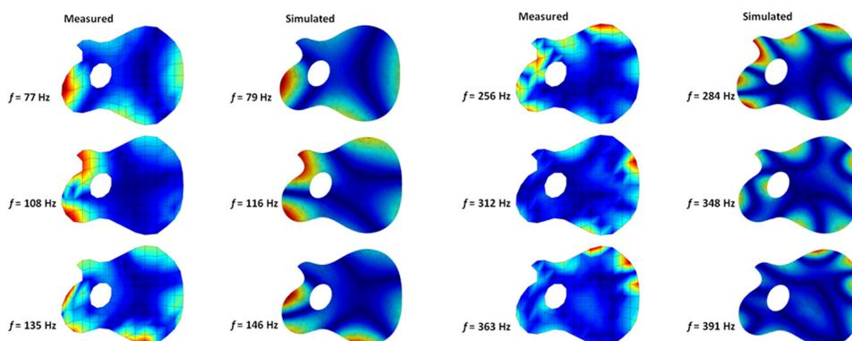
Fig. 3. (Color online) Comparison of measured and simulated modes shapes of the top plate.
