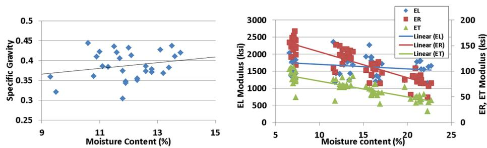
Fig. 1. (Color online) (Right) Sitka spruce modulus of elasticity as a function of moisture content. (Left) Sitka spruce specific gravity as a function of moisture content.
