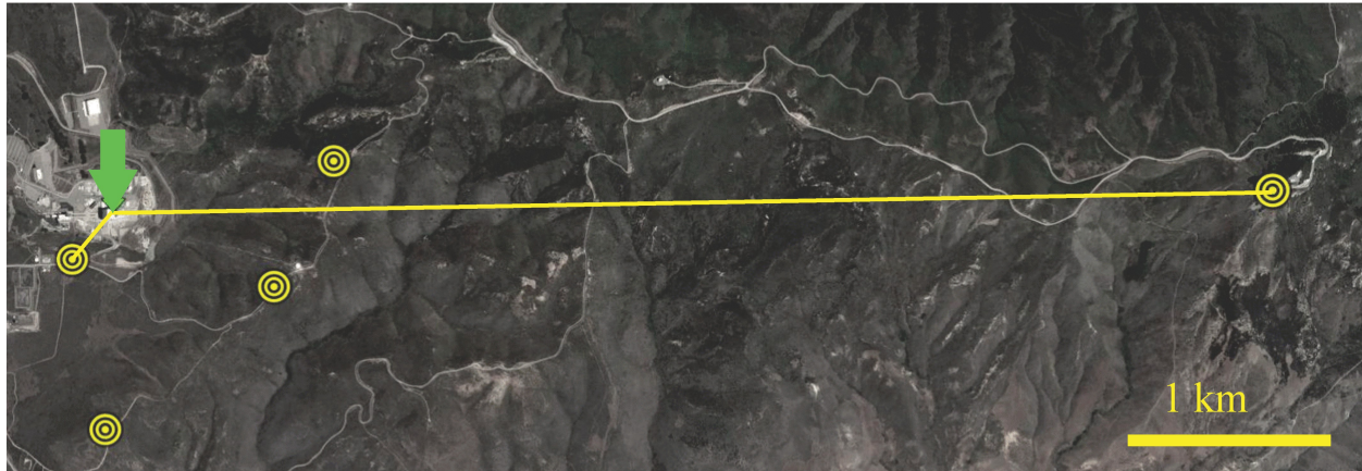
Figure 8: A Google Earth plot showing the location of the mountaintop intensity probe relative to the launch pad. The green arrow shows the launch pad location. The yellow lines show the orientation of both intensity probes. Map data: Google, CSUMB SFML, CA OPC, image ©2022 Maxar Technologies
