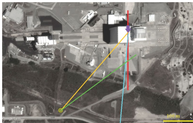
Figure 6: The geometry of the tracking measurement for the close intensity probe. The yellow target indicates the measurement location, and the violet arrow shows the location of the launch pad (under the assembly building). The red line shows the direction of the flame trench. The plume exits along the ground along this line before the rocket lifts off. The blue line indicates the plane of the rocket's trajectory when launched. The yellow line shows the orientation of the intensity probe, and the green line indicates the measured direction of the sound source before take-off, while the jet comes out of the flame trench. Map data: Google, CSUMB SFML, CA OPC, image ©2022 Maxar Technologies
