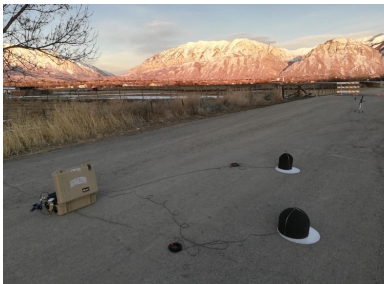
Figure 5. The experimental setup for the outdoor wind noise testing. The two microphone configurations are on the right in the figure, with COUGARxt closest to the camera and COUGAR further away. On the left are the computer and data acquisition hardware. The prevailing wind direction was from right to left in this photograph, with the electronics box being downwind of the microphones.
